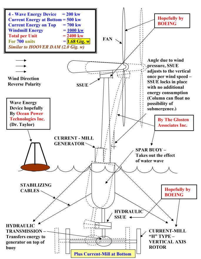
Schematic of Wind/Current-Mill/Wave Energy Plant-©2005-2008 Farid Chouery-all rights reserved Wind is assumed to blow approximately in the same direction (Reverse Polarity) – If wind blows unpredictably, use a vertical column for the windmill and place the SSUE slightly below the lowest point of the windmill fan blade.
